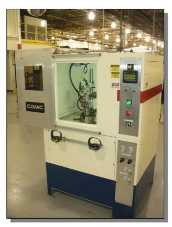
The CDMC-1002 is a member of the 1000 series, and comes standard with an auto-door (with two-hand start switches), an integrated dust collection system, and a touch screen operator interface, as well as dual cutting heads for double sided deburring applications.
